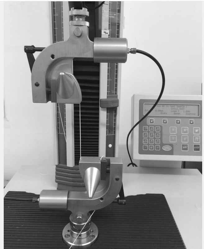
Tensile test of Durus S500 filament according to EN
